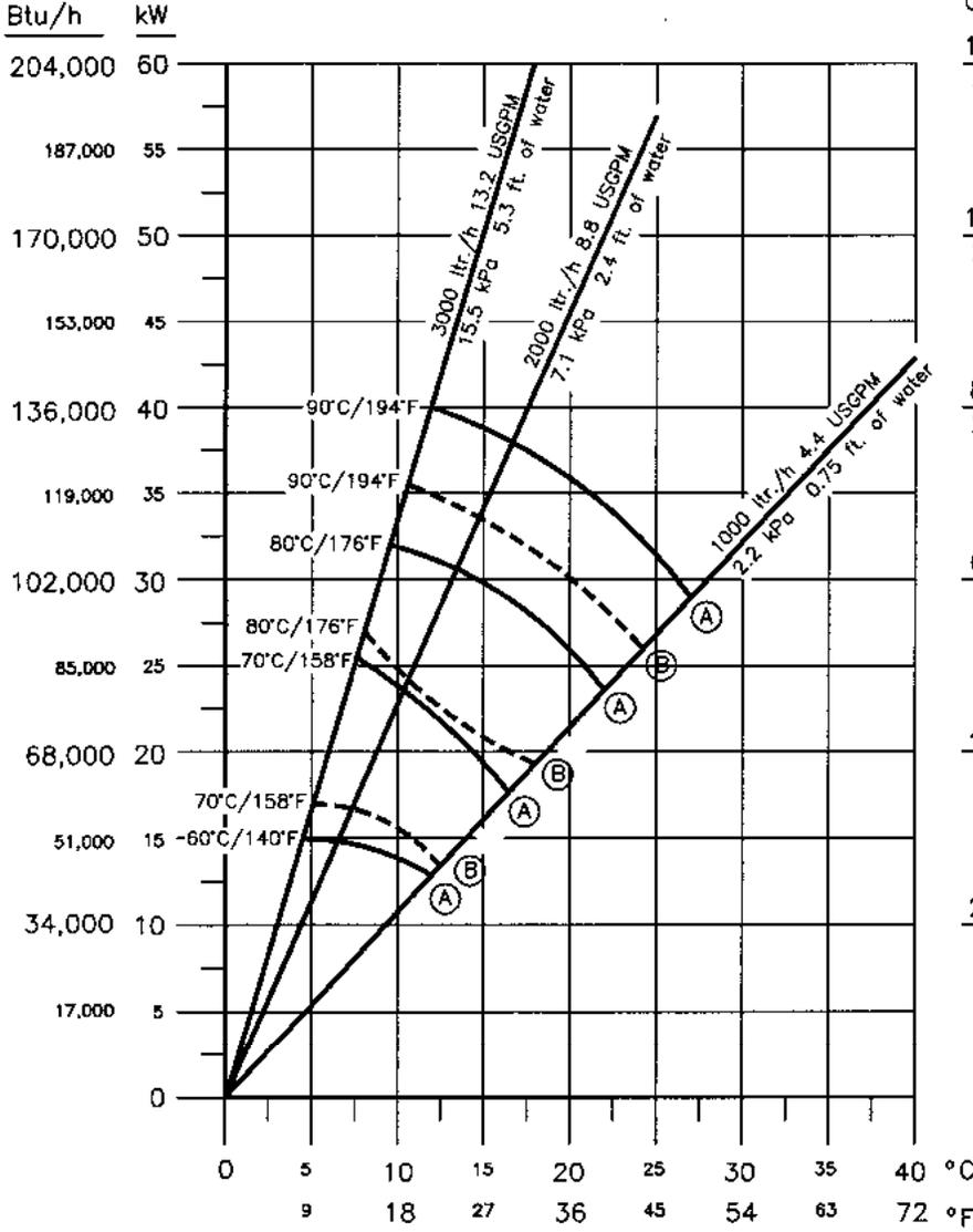
Temperature difference (Boiler supply - Boiler return)
