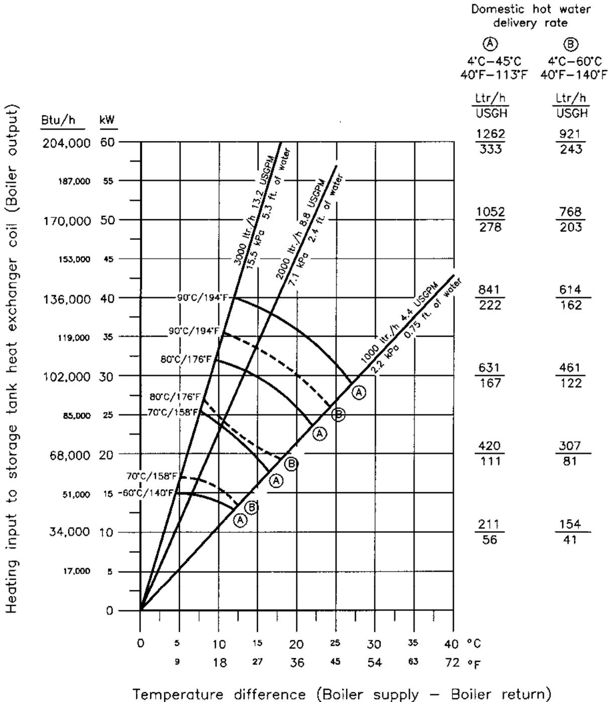
Heating input to storage tank heat exchanger coil (Boiler output)
